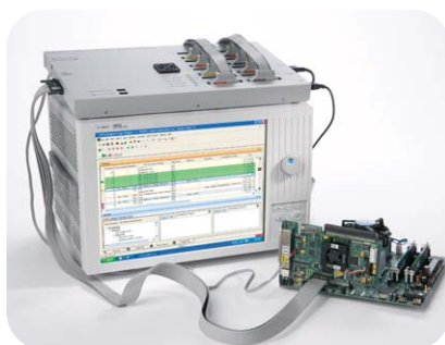
Figure 14. Troubleshoot the transaction and data links of PCI Express buses more economically with the 16800 logic analyzer and the Agilent FSI-60112 packet analysis probe.
