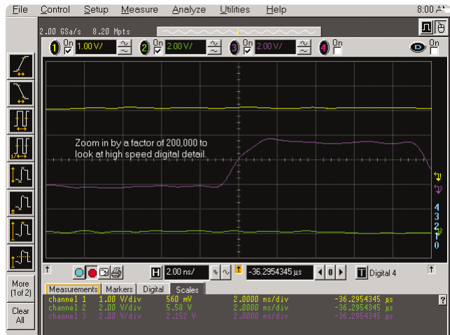
Figure 2. Zooming in by a factor of 200,000: 1 brings the rise time of the SDRAM clock into view.
